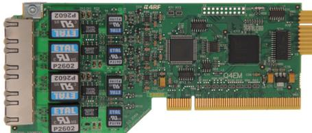
The Q4EM is a quad port analogue interface card providing a 4 wire analogue circuit and single E&M signalling.
