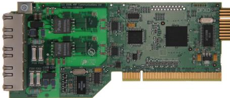
The function of FXO / FXS two wire loop interface circuits is to transparently extend the 2 wire interface from the exchange line card to the telephone / PBX, ideally without loss or distortion. These circuits are known as 'ring out, dial in' 2 wire loop interface circuits. The DFXO interface simulates the function of a telephone.
