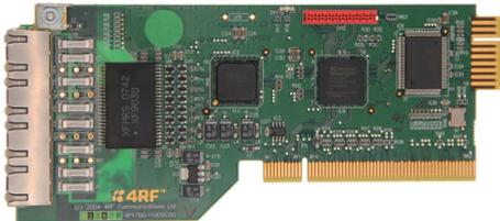
The QJET is a quad port 2 Mbit/s E1 / T1 digital interface providing unframed (G.703) and framed (G.704) interfaces. Unframed (G.703) E1 is typically used for transport of an entire E1 / T1 over the radio link.
