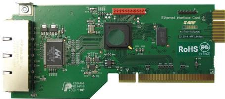
The QETH is a quad port Ethernet interface card supporting 10Base-T or 100Base-TX for transport of user Ethernet traffic. The QETH features are:
