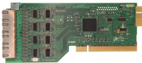
The QV24 is a quad port serial interface card providing asynchronous and synchronous V.24 data transmission.
