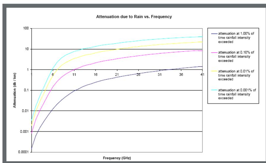
Figure 3: Attenuation vs. frequency for ITU rain climate zone N (35 to 180 mm per hour)
