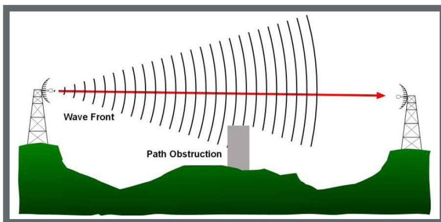
Figure 1: Example of diffraction due to Fresnel obstruction
