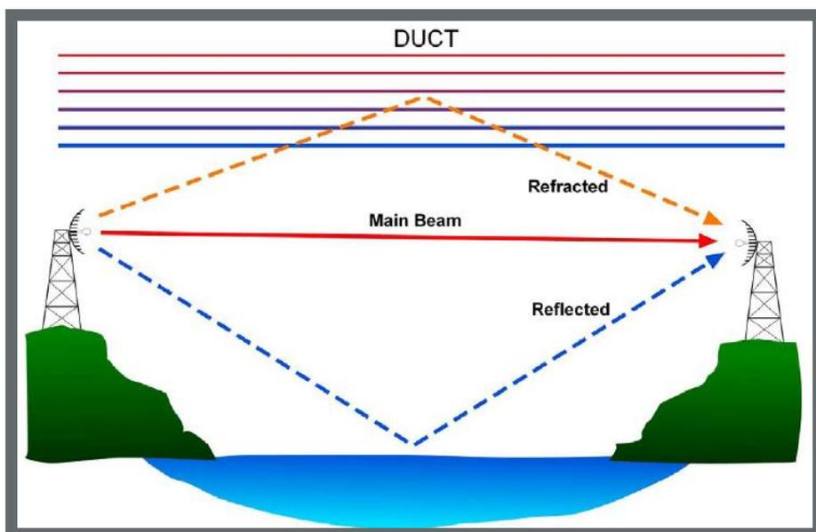
Figure 4: Reflected and refracted multipath
